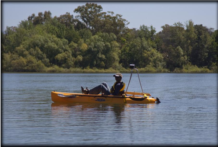
*Figure 6.10:* A pedal kayak used during the long range experiments with the sender rig mounted on the side of the vessel. The elevated housing of the GPS module, the data logger and the wireless communication module can also be seen in this image.
