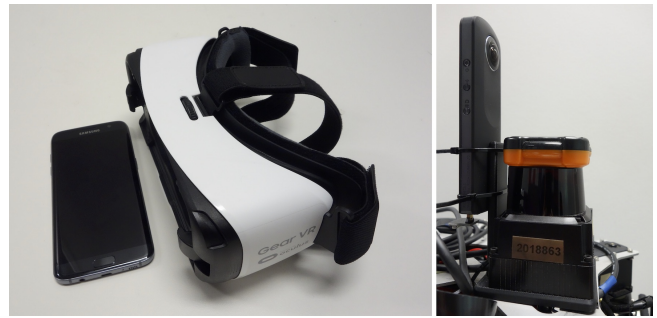
Figure 4: Hardware used; Samsung Galaxy S7 mobile phone with Samsung GearVR (left) and Ricoh Theta S 360° camera with a Hokuyo UTM30LX Lidar (right).
