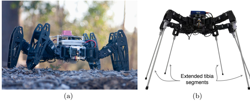
Fig. 1. Modified PhantomX hexapods (a) with additional computing and sensing, (b) with extended tibia segments which reduces its stability during locomotion.
