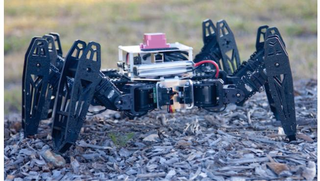
Fig. 1. A modified PhantomX Hexapod robot [7]
