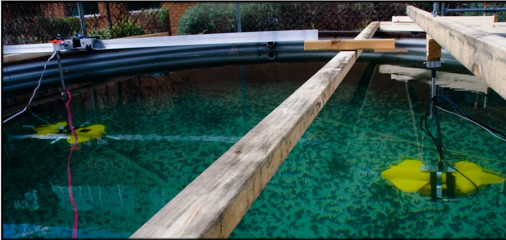
Figure 6.8: Sender and observer rigs attached to the gantry frame placed on top of the test tank. The 3.0m rail and the gantry cart can be seen on the top left side of the image.
