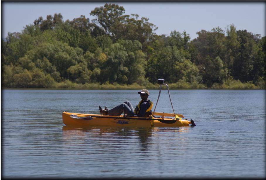
*Figure 6.10:* A pedal kayak used during the long range experiments with the sender rig mounted on the side of the vessel. The elevated housing of the GPS module, the data logger and the wireless communication module can also be seen in this image. [PHOTOGRAPHY BY HIMADHU KOTTEGE]
