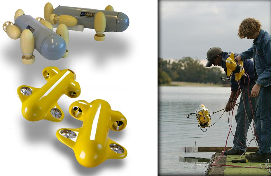
Figure 1.1: Serafina Mk I AUVs [top left], prototype Serafina Mk II AUVs [bottom left] and the author and Jan Zimmer setting up localisation experiments using mock-up hulls [right].
